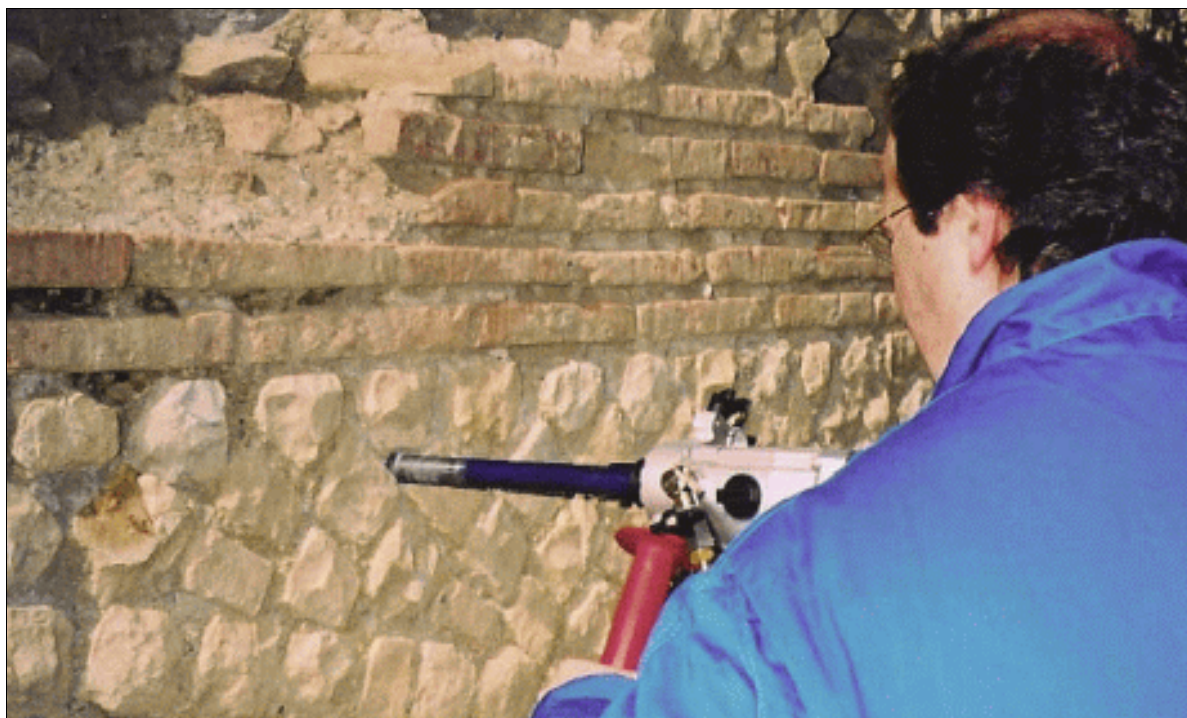
Figure 1 Sampling in Xanten, with a portable wall-driller, equipped with an iron diamond
